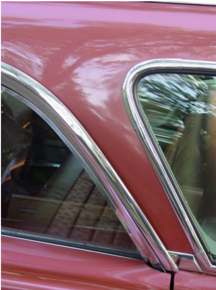
(above) Completely smooth roof panel unique to very early production 1960 Mopar wagons. Later wagons had five embossed ribs for added strength. All New Yorker wagons were built in the Jefferson Ave. plant
