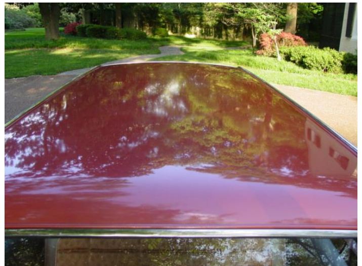
(above) Completely smooth roof panel unique to very early production 1960 Mopar wagons. Later wagons had five embossed ribs for added strength. All New Yorker wagons were built in the Jefferson Ave. plant
