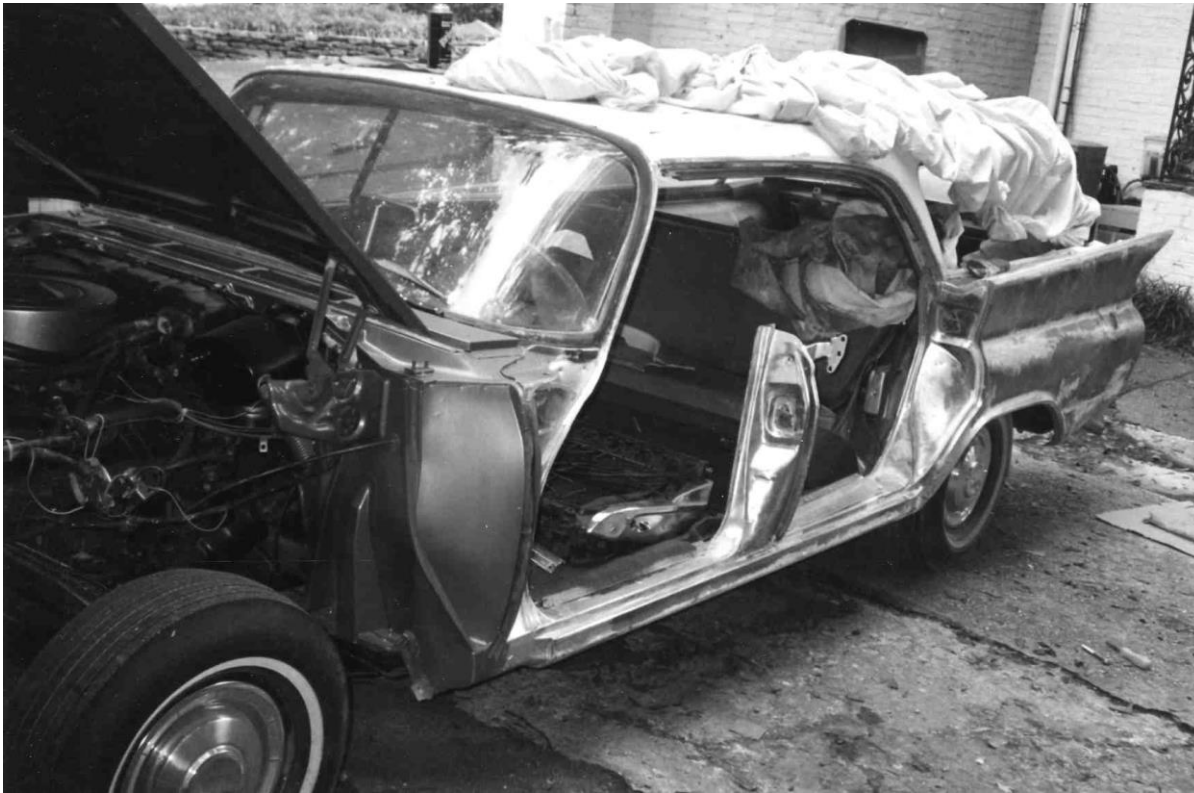
Restoration involved the complete dismantling of interior and exterior. All painted parts were taken to bare metal for refinishing. The cowl, hood and engine compartment had been completed when this picture was taken.
